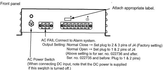
Note: The DC output load must be less than 8A.
